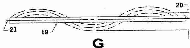
G. LONGITUDINAL WAVINESS (PEAK-TO-VALLEY) 19. EDGE VIEW OF MEMBER 20. PEAK-TO-VALLEY MAXIMUM 21. MEAN CENTER LINE
